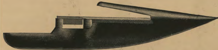
No. 1. Guard finger with our perfect support at rear of scythe, showing how the scythe is held in place and the shear-cut maintained.
