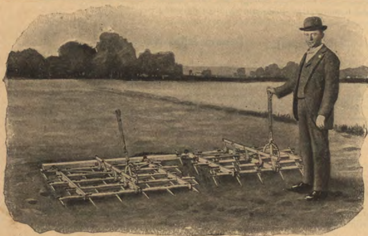
Teeth slanted for transportation; levers in easy reach of the driver.
