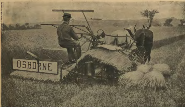
Actual field scene, showing great capacity of elevators and binder. It will not clog. All levers within easy reach of the driver.
