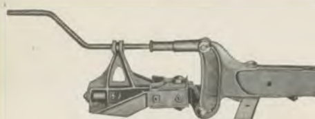
Crank screw device for regulating tilt of the gangs.
