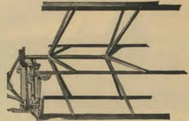
A perfect one-lever, four-motion reel ; light but very strong ; mounted on steel shaft, with two hubs for reel arms.
