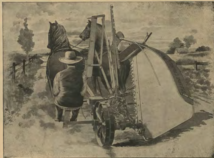
Osborne Columbia Reaper folded for transportation.
