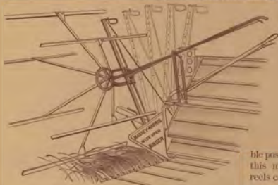
SEE THE COIL SPRING—IT MAKES THE ADJUSTMENT EASY.
