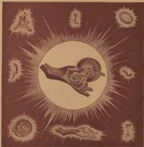
Massey-Harris Twine Knotter, Complete, and also the Parts Comprising it.
