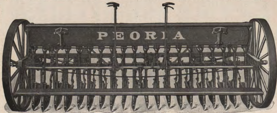
Rear view, 20 x 6" Plain Disc Drill. Double Cover Lid, Double Drive for Feed, Footboard, Strongly Braced. Discs Zig-zagged or Straight as ordered.
