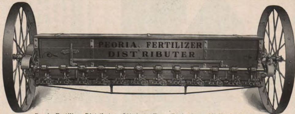
Peoria Fertilizer Distributer—8¼ feet—Force Feed—Sows All Kinds of Fertilizer.
