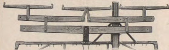
Four-Horse Evener Hitch Changed to Three-Horse Hitch, Pole Set to Side of Drill.
