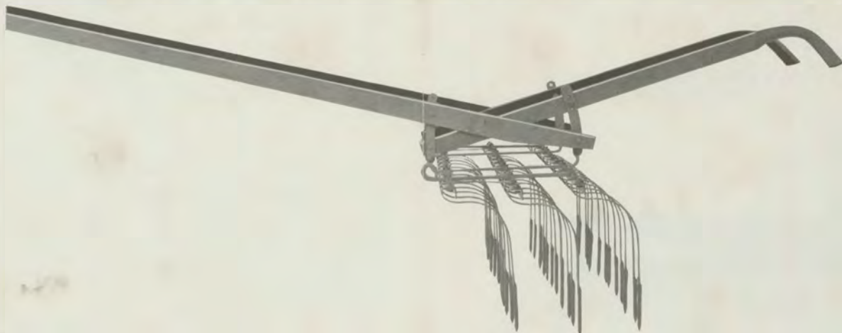
Side View of the Oliver No. 1 Walking Weeder, Showing the Adjustable Handles
