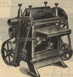
View of Feed Side Showing Double-gear'd Machine with all Four Feed Rolls Driven
