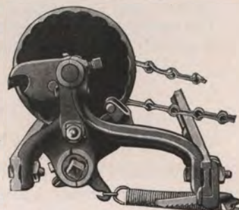
The clutch in operation. The little roller on the dog coming in contact with the grooves eliminates wear on both the dog and the ratchet
