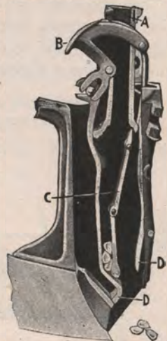
The kernels dropped in the hill. Observe that D has moved downward, forcing the corn out in a bunch
