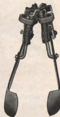
Covering shovels for planters with double disks
