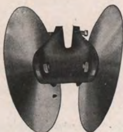
Rear view of double disk furrow opener attachment. Note the simple method of attaching
