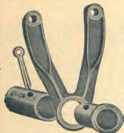
To Show Secure Fastening of Tooth-Bar.
