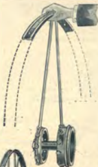
Section of the Osborne Double Hub Bicycle Wheel; 20 Spokes.
