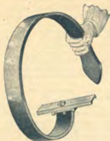
Another Tooth Fastening—all the strain on the bolt.
