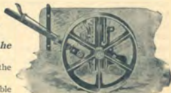
Easy and convenient Raising and Lowering Device for Grain Wheel.
