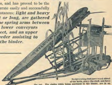
Powerful reciprocating jaws to force the cut and convey the butts. No corn pulled up by the roots. No winding with weeds.
