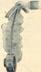
Section of the Single Hub Wheel Used on other Rakes; 12 to 16 Spokes.
