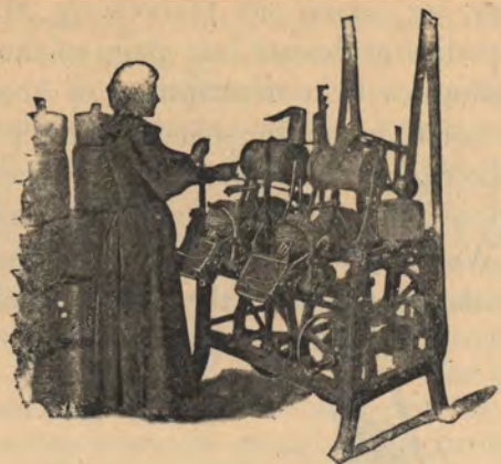
A. Ealling Machine that winds 1000 feet of Twine every minute.
