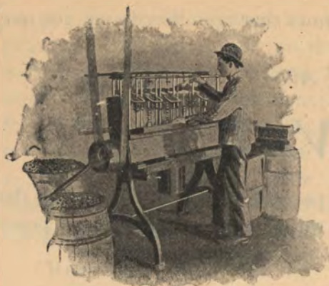
A Five Spindle Nut-Threading Machine in the Osborne Works.
