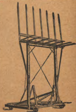
Adjustable Arm Stacker at its Lowest Height with Lifting Bars Disconnected
