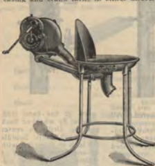
No. 45 Champion Lancaster Geared Direct-Drive Agricultural Forge. Hearth 22 in. in diameter, fan 10 in., with shield, weight 115 lbs. .... $10.15
