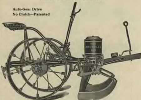
Janesville No. 7 Planter—Gear Drive, Shoe or Stub Runners Our Regular Planters are made in 30" and 36" Wheels
