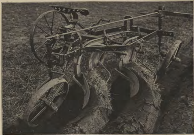
Wonderful picture of Janesville Gang with S. & S. Bottoms, just as the camera saw it. Note the folding process of the furrow. The S. & S. Bottom does not pitch the furrow.
