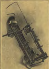
Showing Frame, Wheels and location of Pole and Seat. Forty Inch Wheel, Roller and Brass Bush Bearings. Main Drive Gears. Cutting Apparatus. Conveyor Fingers. Adjustable Chain Tighteners. Separate Idler Sprocket Box. Binder Attachment. Automatic Gates. Set for Short Corn.
