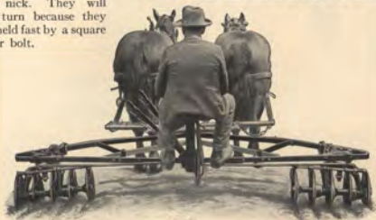
Showing the wide Extension Frame attached to regular Diamond Frame.
