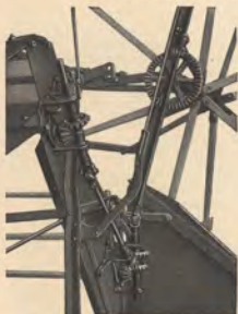
Lower portion of the 51-inch reel standard. Also the gearing.
