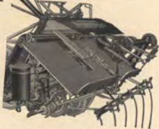
For very long grain End Board Piece is removed. View also shows panel removed to permit easy oiling of Binder parts.
