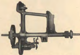
The strong, one-piece Main Frame of the bridged type. Also shows the Automatic Throw-out and Roller Bearings.
