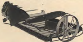
Showing grain wheel and both inside and outside dividers folded out of the way.
