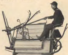
The elevators and convenient levers. The large roller at the bottom of upper elevator prevents choking.
