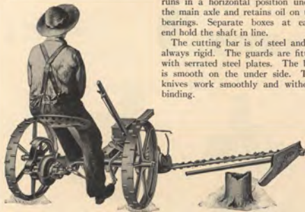
The use of a convenient Foot Lever permits the clearing of field obstructions. This is a view of the No. 10 Mower.
