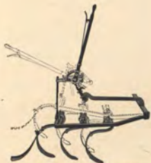
Showing range of adjustment of the spring teeth.
