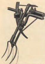
Fork Spring Trip, which enables it to easily spring over any field obstruction.
