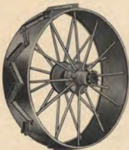
The main or master wheel, 10 inches wide. Note the position of the calks.
