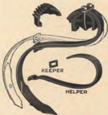
View of spring tooth showing detail of the keeper and helper.
