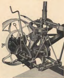
Suspension Bar; Tilting Lever; Bevel Gear and Spur Gear; Automatic Trip; Clutch Shifter; Platform Support Plunger Crank.
