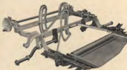
Showing the front truck axle bearing and fastening.
