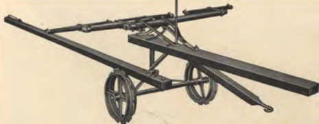
View of tongue truck which is easily and quickly attached to all Johnston Binders.
