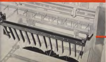
● The NEW IDEA Lime Spreader, showing position of discs, rake and drive chain.
