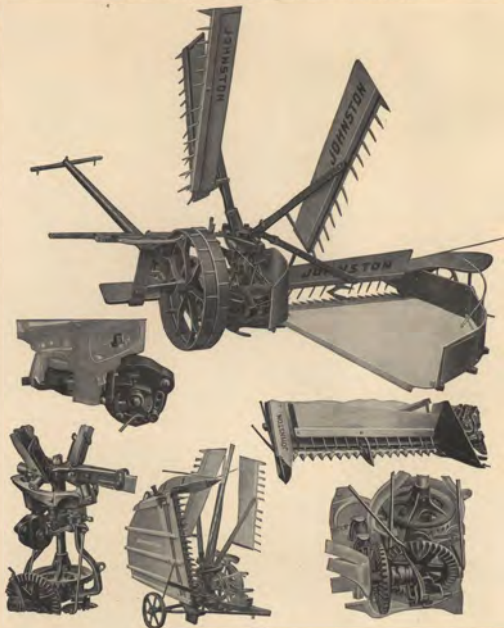
Rake Standard. Automatic Trip. Reaper folded. Rake parallel with bar. Reaper Gearing.
