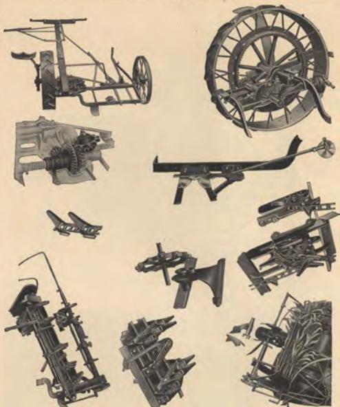
Showing Frame, Wheels and location of Pole and Seat. Forty-inch Wheel, Roller and Brass Bush Bearings. Main Drive Gears. Cutting Apparatus. Conveyor Fingers. Separate Idler Sprocket Box. Adjustable Chain Tighteners. Binder Attachment. Automatic Gates. Set for Short Corn.
