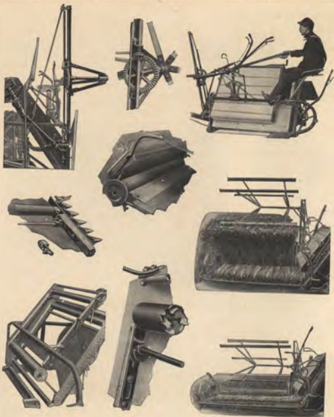
Reel Standard and Gearing. Convenient Levers. Canvas Tighteners. Seventh Roller. Elevator showing Rollers. Elevator Canvas Tightener. Reel set for tall and short grain.
