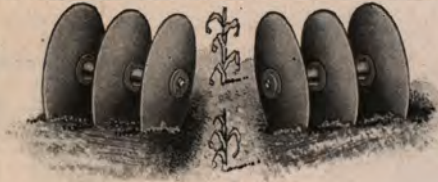
Discs Set to Throw the Soil From the Row in Listed Corn
