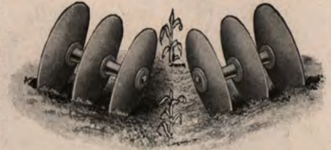
Discs Set to Throw the Soil From the Row
