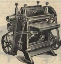
View of Feed Side Showing Double-gearred Machine with all Four Feed Rolls Driven
