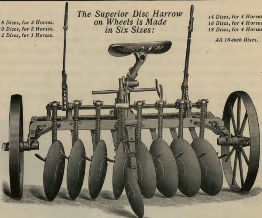
REAR VIEW SHOWING COMPACT CONSTRUCTION OF CENTER DISCS.
