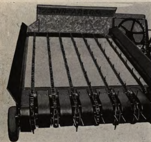
Fig. 2. Front View Pick-up Unit. Full floating—Balanced off main axle.
