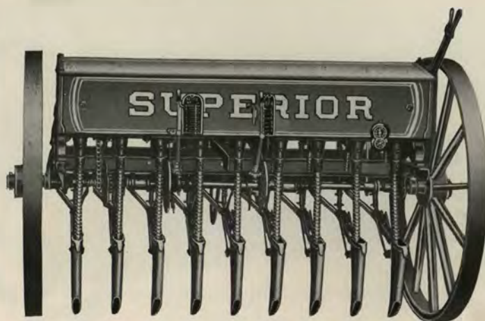
Superior 9 x 7 Spring Hoe Fertilizer Drill With Steel Ribbon Tubes.
