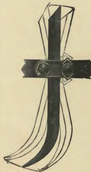
By changing each Tooth Clip, the Pitch of the Teeth can be easily Adjusted Forward or Back
