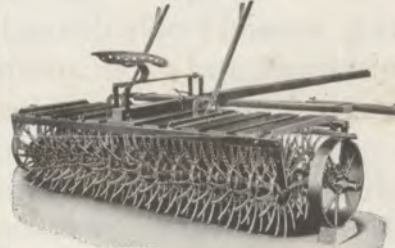
Illust. 23. McCormick-Deering 2-row rotary hoe. By getting young weeds before they come up, it usually saves one or more cultivations. It can be used on the seed bed any time after plowing and until the crop is 8 inches high. It also is the ideal soybean cultivator. Supplied in a variety of sizes for horse and tractor use.
