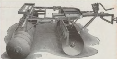
Illust. 12. McCormick-Deering No. 5 tractor disk harrow especially suited to light soils. Available in 5, 6, 7, and 8-foot sizes. Disks 16 or 18 inches in diameter are available.
