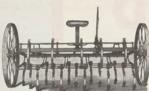
Illust. 19. McCormick-Deering field cultivators continue to grow in popularity for summer-fallow work and for weed eradication. Equipped with spring teeth, as shown here, they do a good job in quack and Johnson grass, cultivating many acres a day. Supplied in 6, 7½, 9, and 12-foot sizes. Wide variety of shovels available.
