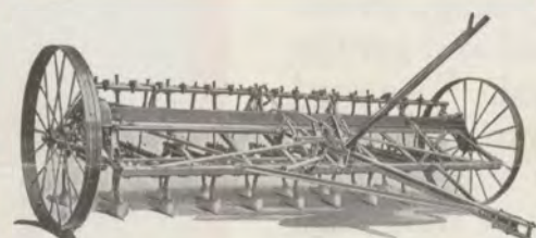
Illust. 20. McCormick-Deering stiff-tooth field cultivator equipped with power lift and depth regulator. This combination brings the gangs amply high above the ground for transporting, regardless of the depth of penetration set by the regulator.
