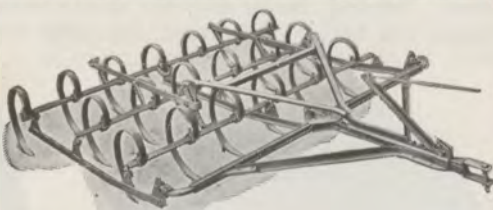
Illust. 9. McCormick-Deering 2-section, self-clearing tractor spring-tooth harrow available in sizes from 4½ to 16½ feet. The position of the teeth is controlled by a rope from the tractor seat.
