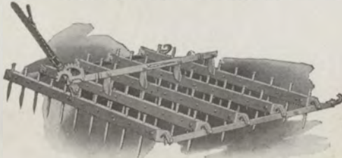
Illust. 7. A McCormick-Deering wood-bar lever harrow section. Wood-bar harrows have ample weight to assure good work in cloddy ground. One to 4-section sizes, with 41 teeth to the section.
