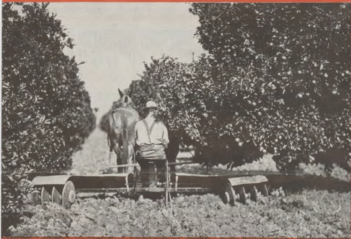
Illust. 2. Low, overhanging branches are not damaged when this McCormick-Deering adjustable-width orchard disk harrow with sheet-metal shields is used. The McCormick-Deering tillage line includes a wide variety of tools for use with horse or tractor power.
