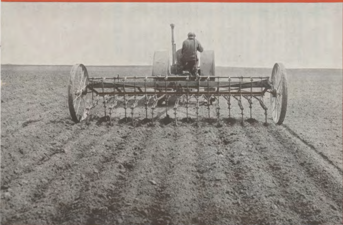
Illust. 3. McCormick-Deering field cultivators, originally used only in summer-fallow regions, now are becoming popular elsewhere for doing a quick, thorough job of removing quack grass, Johnson grass, and similar weed pests. Three times over with a field cultivator usually costs no more than once over with a plow.
