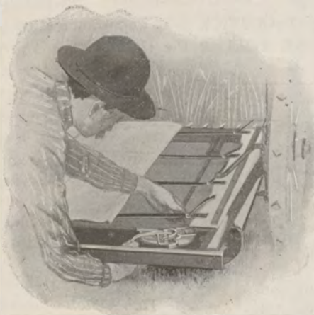
Throw the Lever In. This Tightens the Apron
