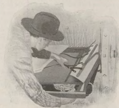
Throw the Lever Out. This Loosens the Apron
