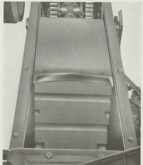
The Shear Plate, Plunger and Plunger Slides, which slice and compress the Bales made on the "Automaton."
