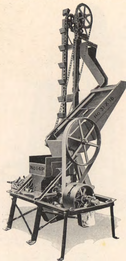
NO. 14P PULVERIZER EQUIPPED FOR MAKING OYSTER SHELL GRIT
