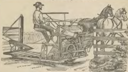
Triumph No. 7, Wood Frame Binder, 5½ ft. cut. Folded to pass through a 10 ft. gateway.
