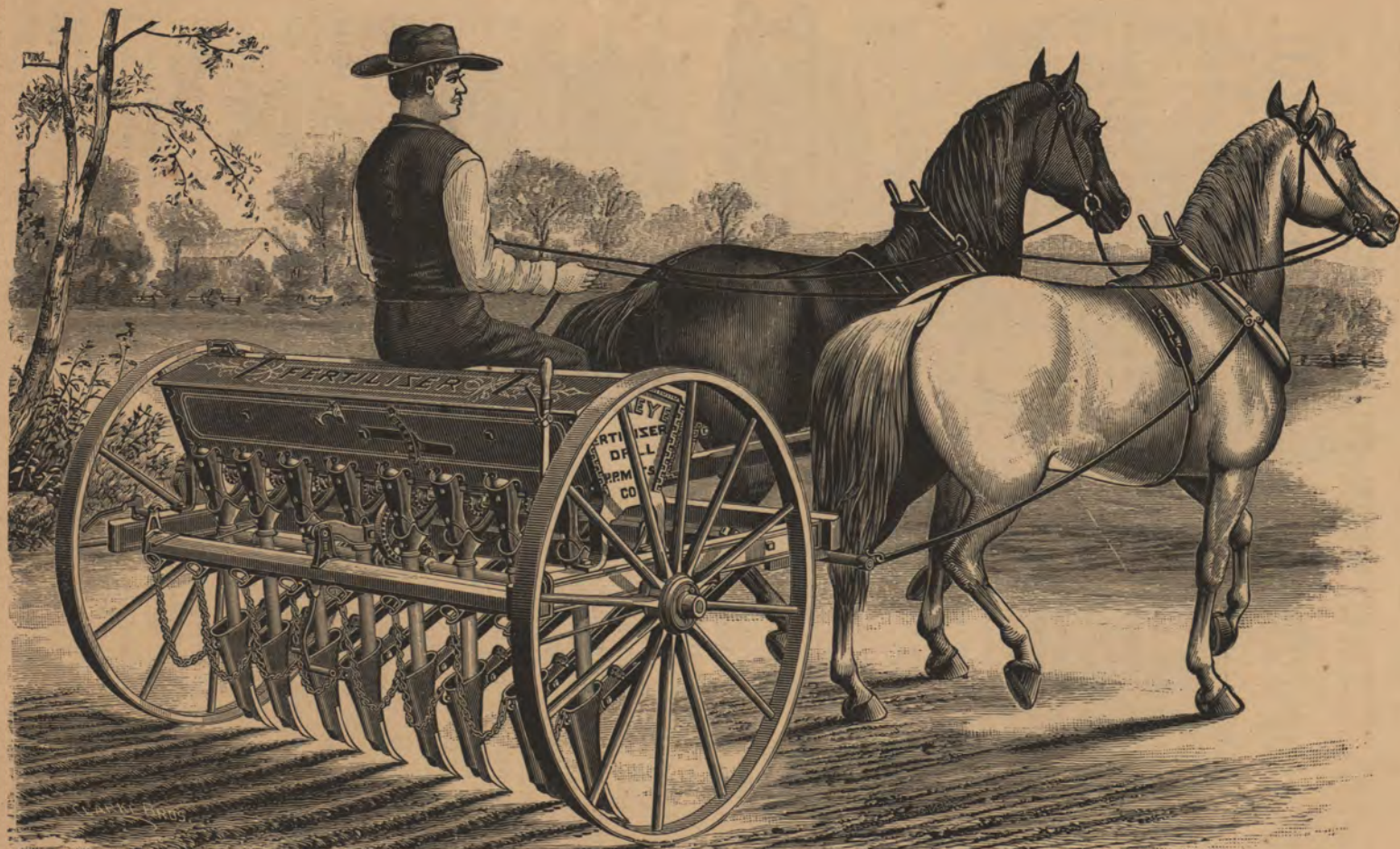
THE NEW IMPROVED BUCKEYE COMBINED DRILL AND FERTILIZER.
