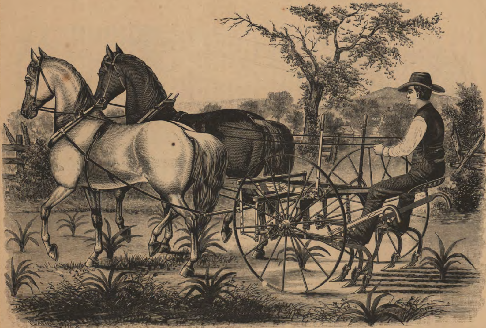
THE NEW NO. 8½ BUCKEYE SUNBEAM, COMBINED RIDING AND WALKING CULTIVATOR. Manufactured by P. P. Mast & Co.
