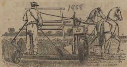
The above Cut shows how, with a steady team, one man can both Rake and Drive on the John H. Manny Machine.
