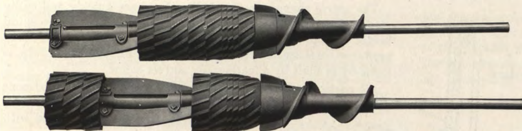
Two Views of Shelling Cylinder and Spiral Force-Feed. The Upper for Husked Corn, the Lower for Snapped Corn
