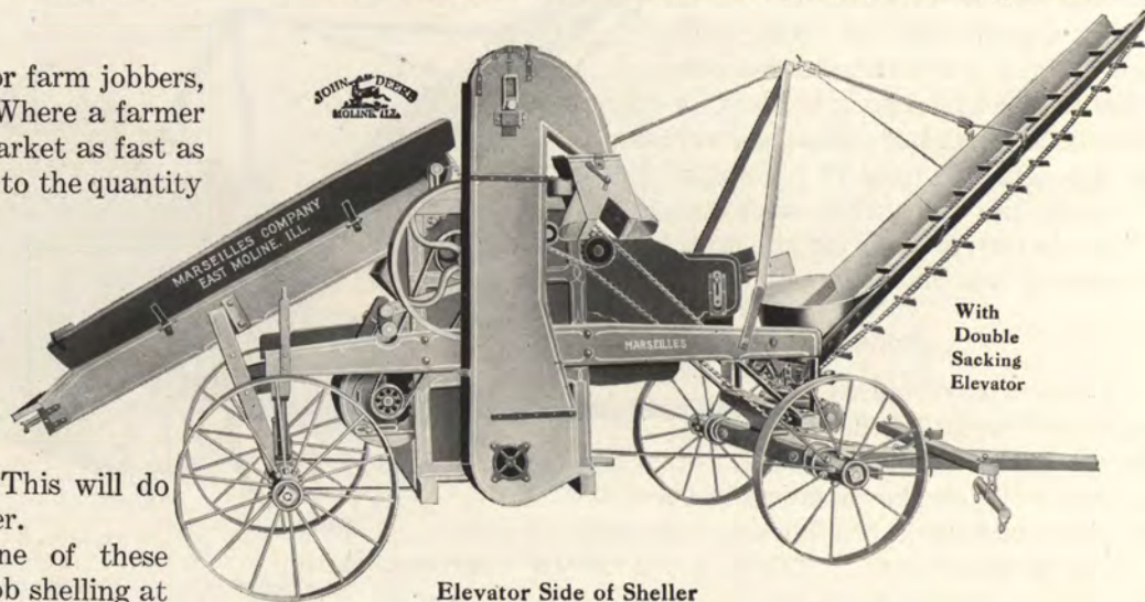
Elevator Side of Sheller
