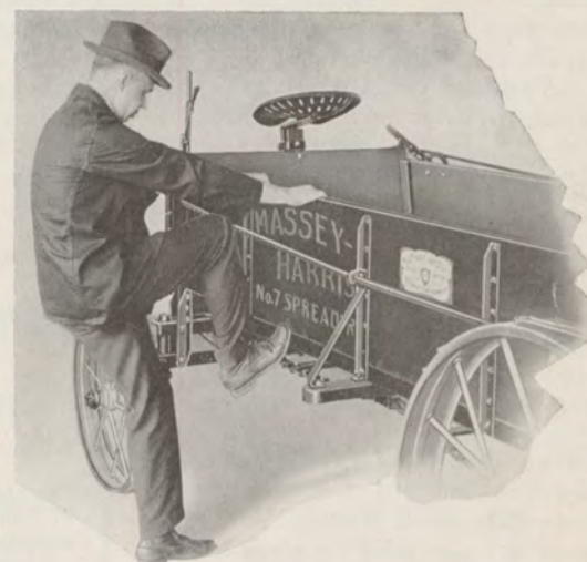
You can't make the sides of the box spread apart. They are braced like those of a wagon.
