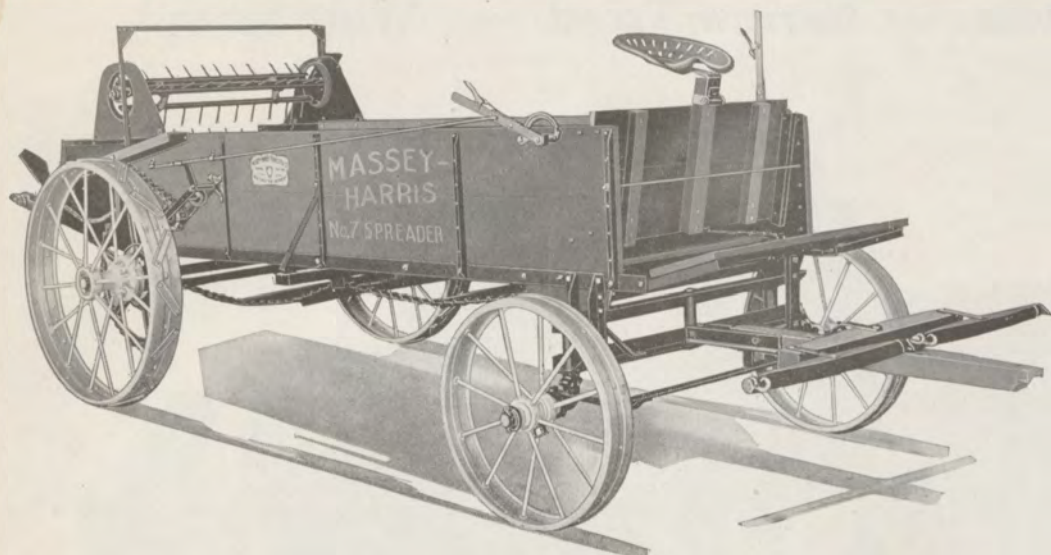
The machine viewed from the right front corner. Note the accessibility of the two levers and that the front and rear wheels track.
