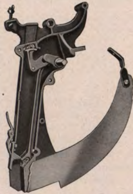
Superior Plain Runner Post with side piece removed showing valves closed.
