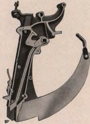
Superior Plain Runner Post with side piece removed showing valves set for drilling
