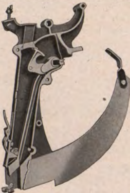
Superior Plain Runner Post with side piece removed showing valves open.
