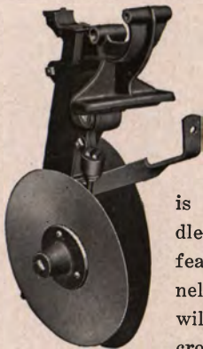
Superior Double Disc Furrow Opener
