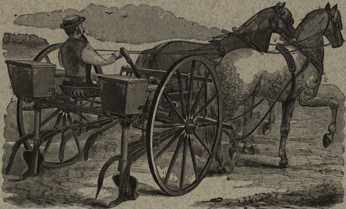
View of Machine Rigged for Planting Corn with Phosphate Attachment.
