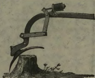
Position of Spring Hoe when passing an Obstruction.
