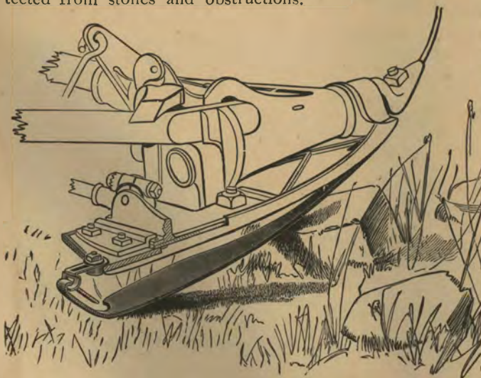
Supplemental Shoe on the Deering Mowers.
