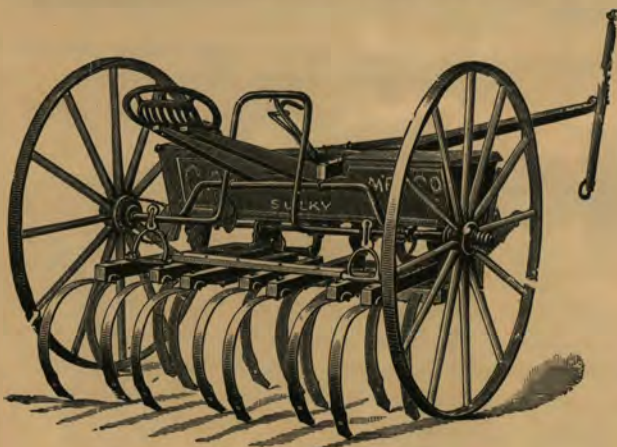
New American Harrow with Grain Seeder Attachment, Arch Lever, Wood Wheels, Flat Teeth.
