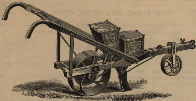
8.—THE EVANS ONE-HORSE SOLID WHEEL CORN DRILL AND FERTILIZER ATTACHMENT.
