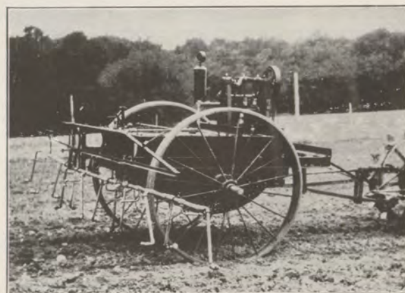
No. 6063 Power Take Off Sprayer Three 2\frac{3}{4} " Cylinder Pump. Develops 400 lbs. pressure with 6 row, 18 nozzle boom or 2 spray guns
