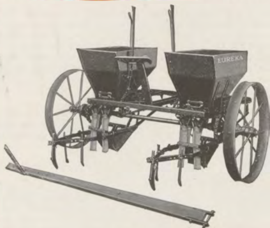
Eureka No. 172 Two-Row Fertilizer Distributor (Weight 500 lbs.)
