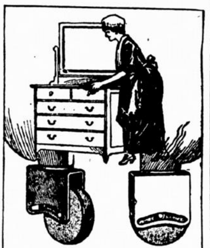
Caster That is Central Under Leg of Furniture When at Rest, but Moves to One Side When Rolled.
