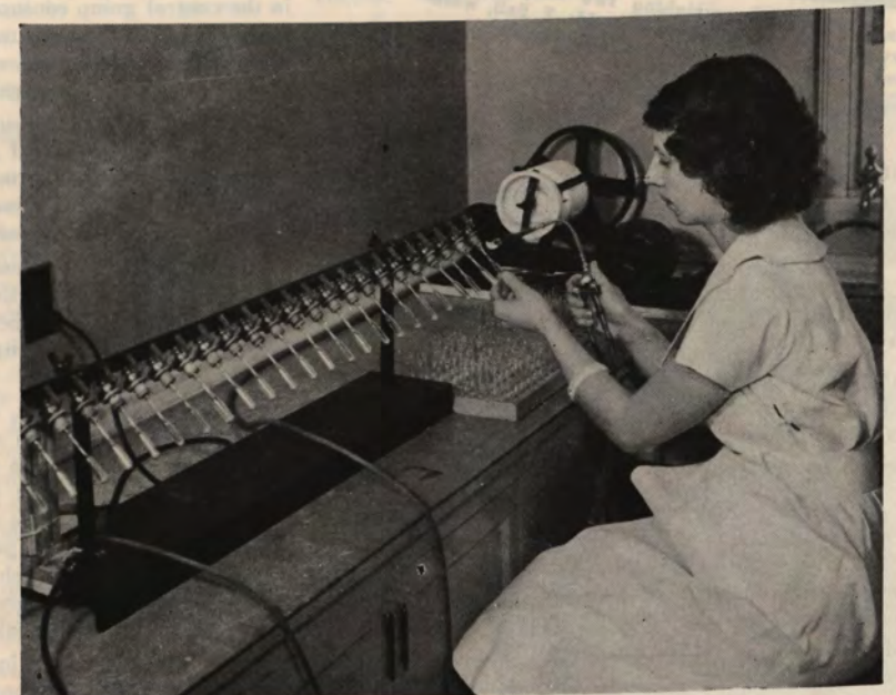
Fowl Laryngotracheitis Vaccine is shipped in vacuum sealed vials. The above picture shows this operation. Throughout the entire production of Dr. Salsbury's Vaccine extraordinary care is taken to protect it from contaminating germs. Now that the finished product is being prepared for shipping it is packed in vacuum sealed glass vials to maintain this purity and potency along its route to the ultimate user.
